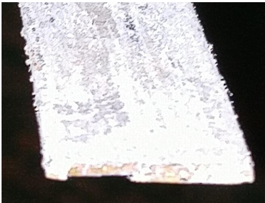
Figure 3 – Pitting corrosion of the stainless steel cathode during NaCl electrolysis.
